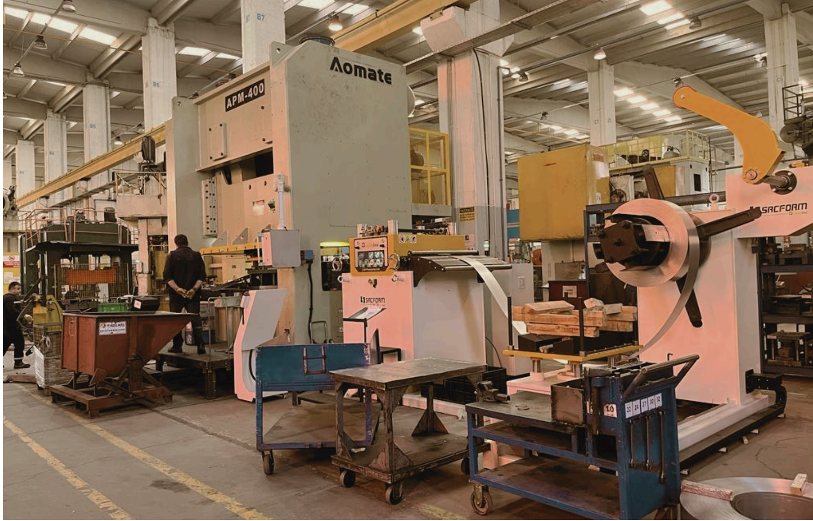
PRECISION PRESS APM-400 TON (1200 X 1600 1200 X 1600) and ROLL SHEET DRIVE
