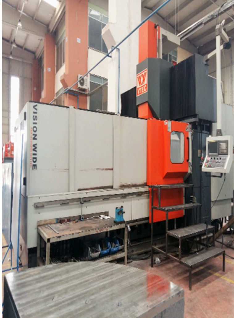
VTEC 3 Axis Bridge Type CNC Machine (x:2450/y:3450/z:900)
