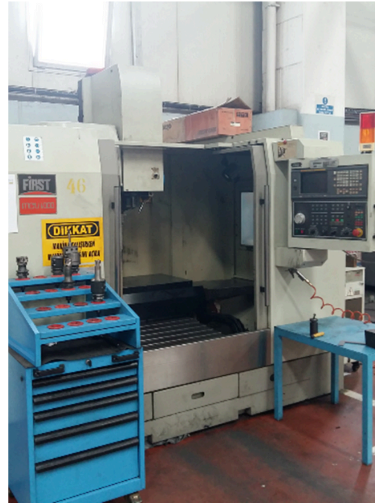
FIRST MCV 1000 3 Axis CNC Machine (x:1000/y:500/z:500)
