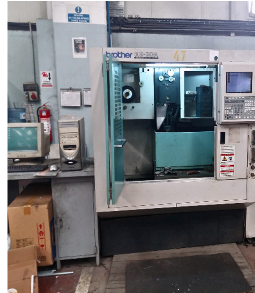
BROTHER HS-50A 4 Axis Wire EDM Machine (x:420/y:260/z:160)
