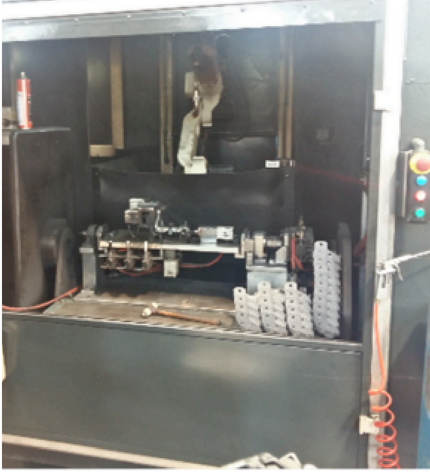
GAZ ALTI KAYNAK ROBOTO 350 A DAIHEN (1 Adet)
