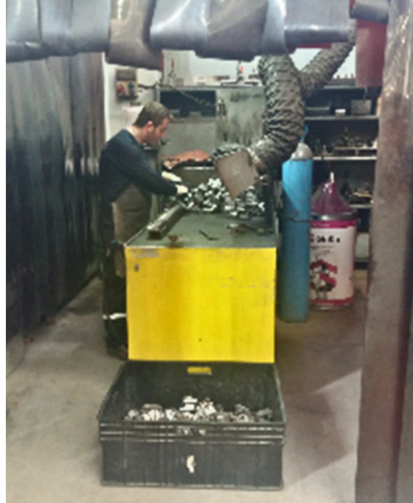
GAZALTI KAYNAK TEZGAHI 1.2 mm Tel / 320-500 A ARCTECH (3 adet) GEDİK FRONIUS (1 adet) EXPRESS WELD (1 adet) TURALLAR (2 adet) DAIHEN (1 adet)
