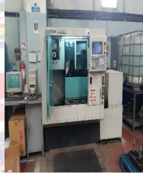
BROTHER HS-50A 4 Eksen Tel Erozyon Tezgahı (x:420/y:260/z:160)
